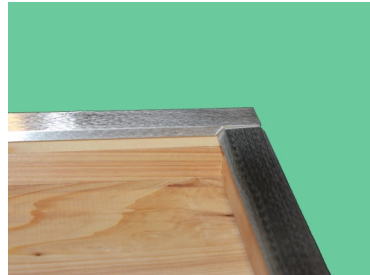
Fig. 3—End Rail Placement Standard bottom board shown
