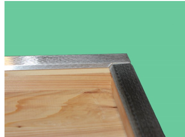
Fig. 3—End Rail Placement Standard bottom board shown
